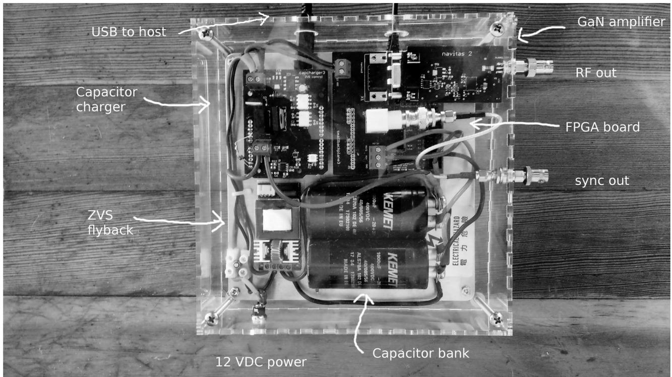
Fig.2 Single channel pulser
