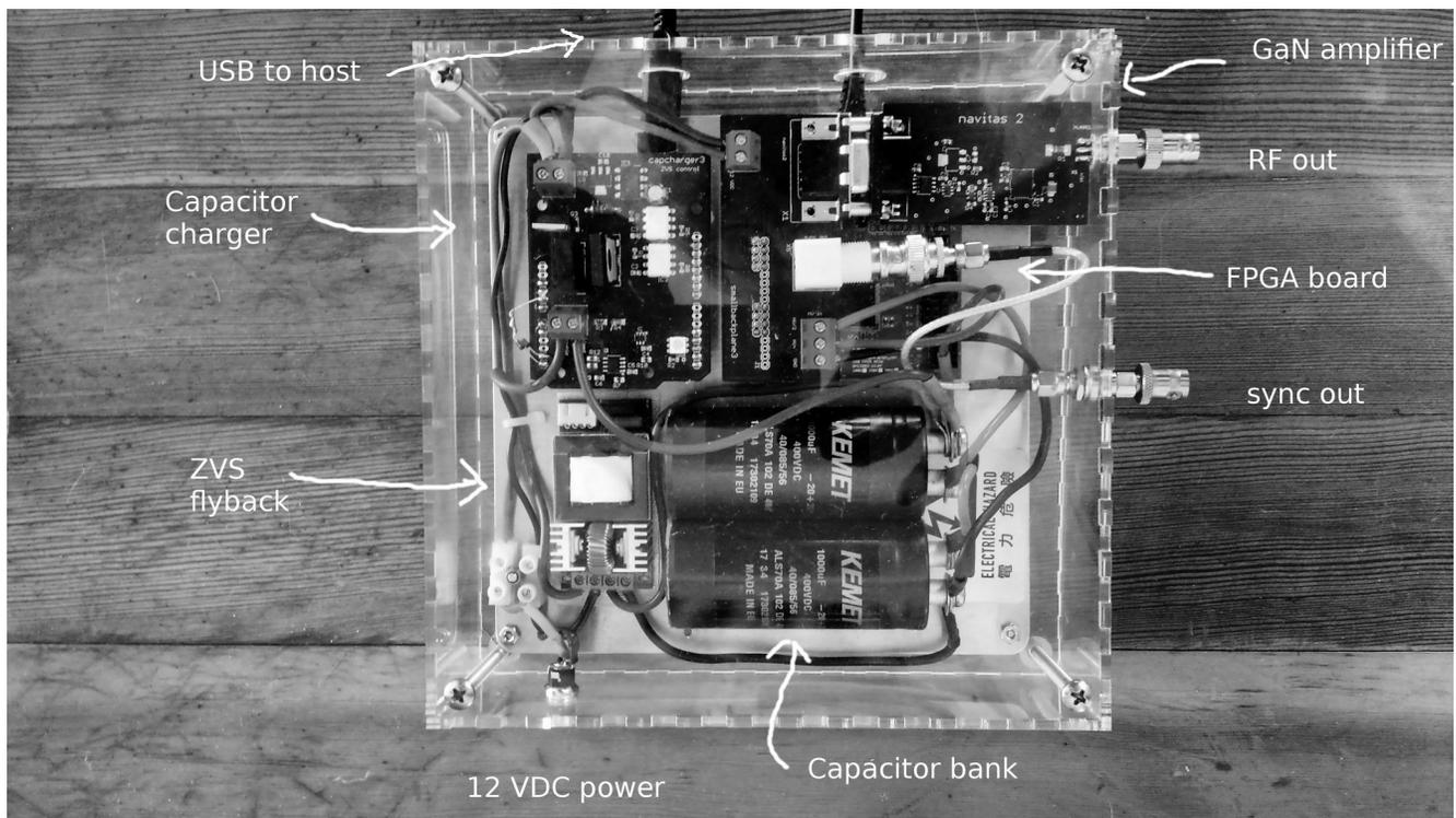
Fig.2 Single channel pulser
