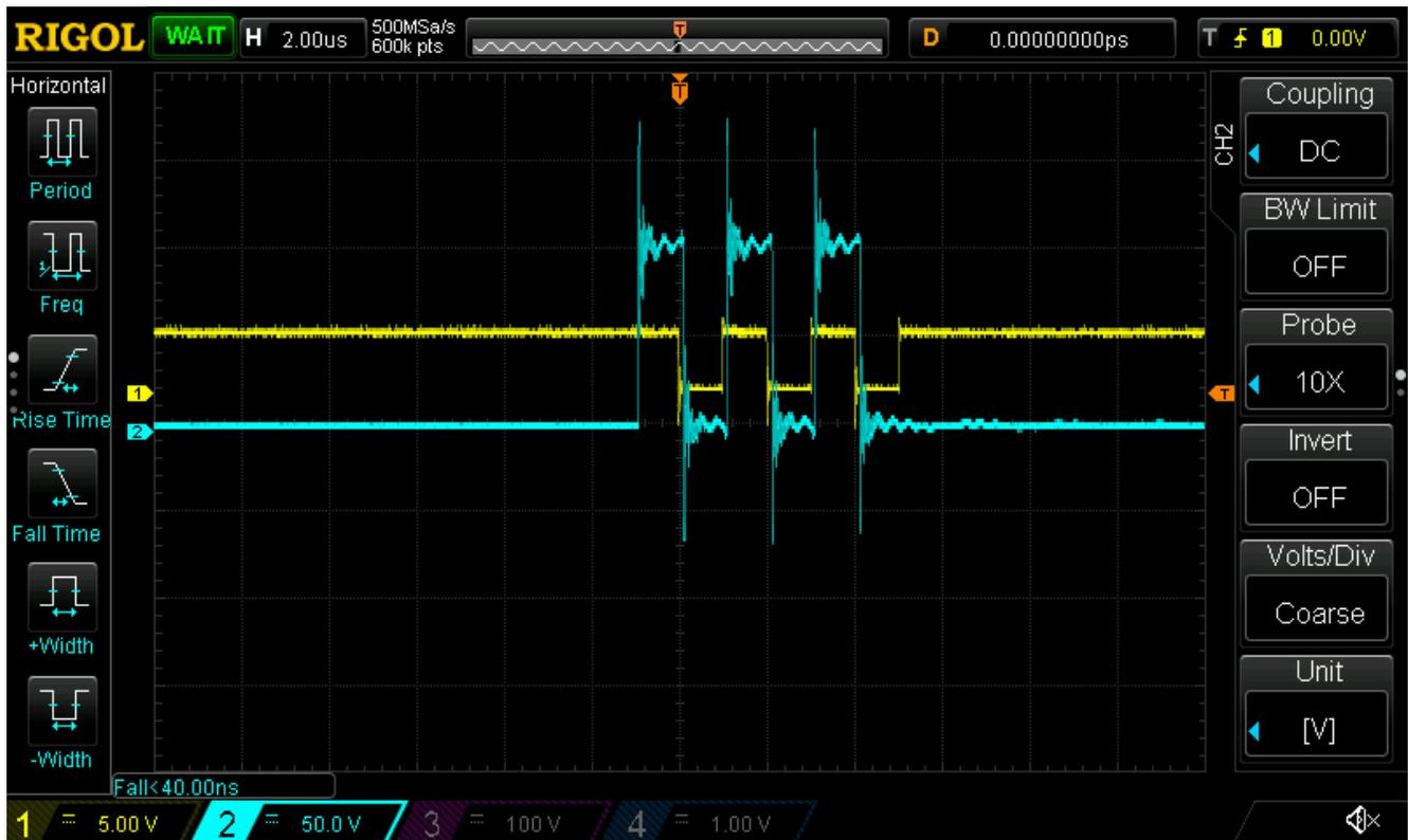
Fig.4 Burst of 3 cycles into HIFU transducer at 100 Vpp (blue)
