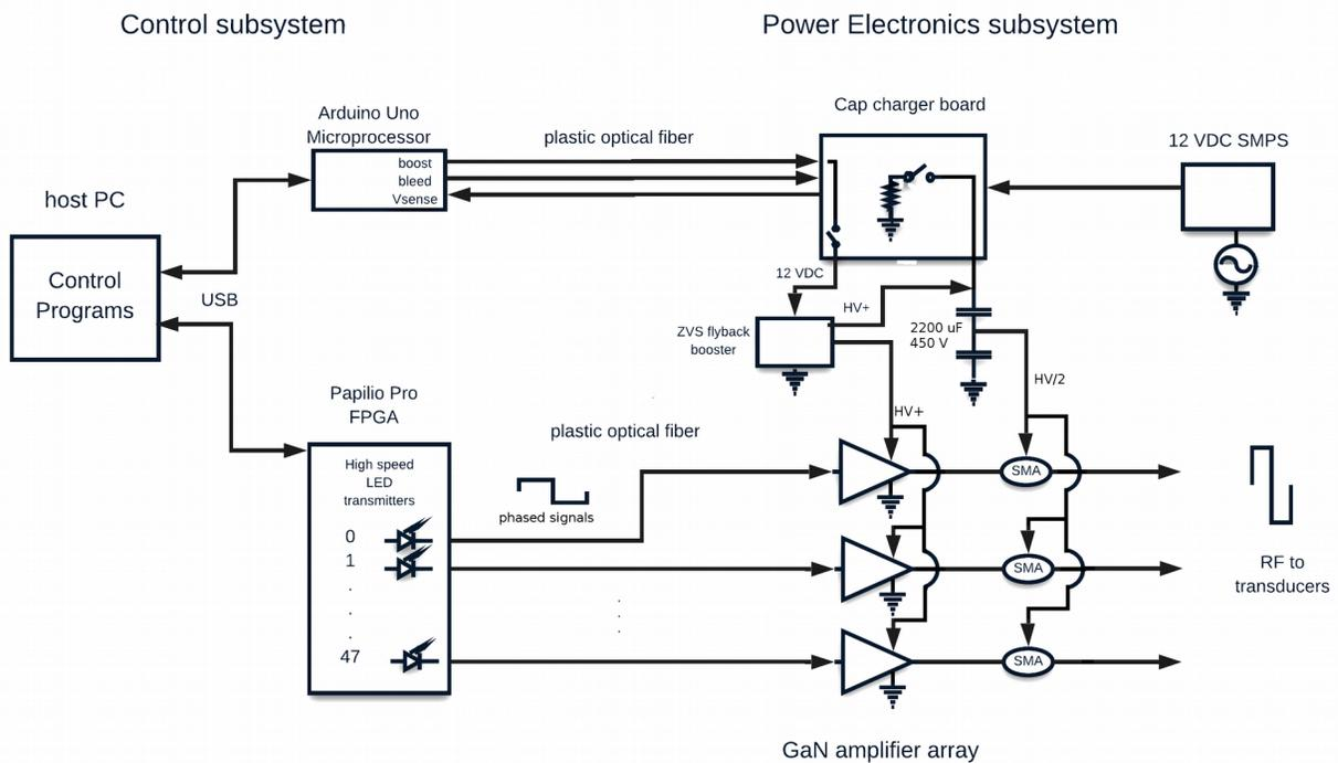
Fig.1 Pulser Mark 5 Architecture
